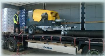
Used Selwood S300 sold to a customer in Finland. The 12" automatic self-priming unit is capable of flow of up to 1200m3/h and is housed in a full sound attenuated box canopy reducing sound levels to at least 60dBA at 7m. The set was fully checked and tested at our workshop facilities in Shorpham and re-painted Red prior to sale.
